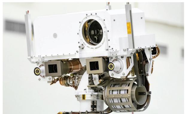
The head of Mars 2020's remote sensing mast which contains the SuperCam instrument (its lens is in the large circular opening). In the gray boxes beneath mast head are the two Mastcam-Z imagers. On the exterior sides of those imagers are the rover's two navigation cameras
